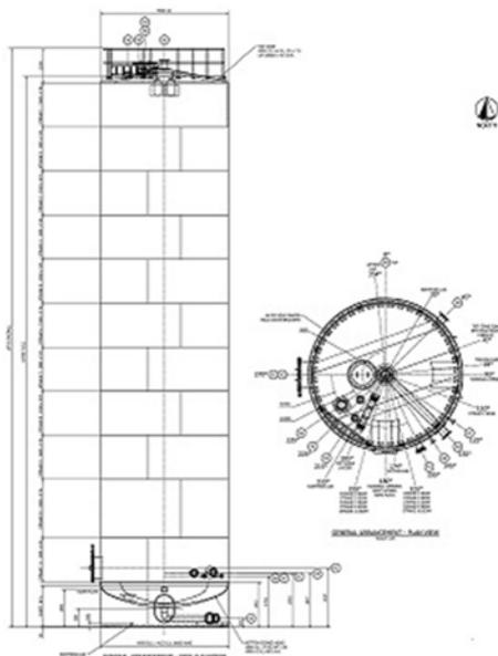
All elements of design considered Australian and International standards to optimise the life and performance of each tank. Structural design considered the density of stored fuels - diesel and ULP, along with the venting requirements for petrochemicals, in accordance with AS1692. Additional components were added to each tank; these included access points for maintenance and internal floating roof systems to create vapour barriers.
